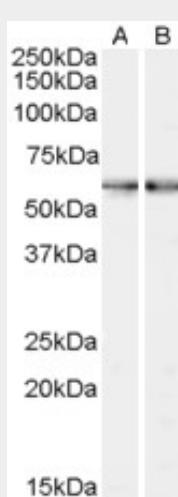
A) AF2009a and B) AF2009b (0.3 µg/ml) staining of Human Bone Marrow lysate (35 µg protein in RIPA buffer). Primary incubation was 1 hour. Detected by chemiluminescence.
